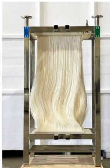
Advanced Ultrafilter (UF) Membranes – Absolute Barrier to Suspended Solids & Micro-organisms
