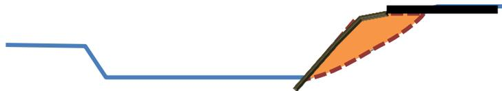
Channel is excavated (too wide) and flood generated sediment is used to shore up road shoulder, road is remade and stream bank is armored.
