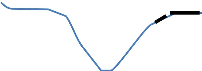
Almost immediately, and often during the same event, the impinging flows of the incised stream channel erode the embankment and the bank armoring and road with it.
