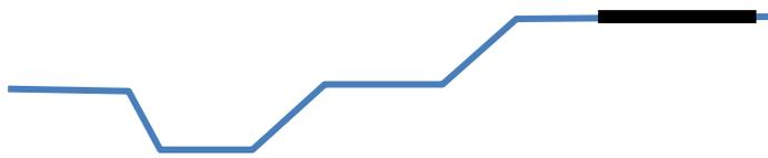
Pre-flood stream channel / floodplain cross-section with road surface depicted on an upper terrace to the right.
